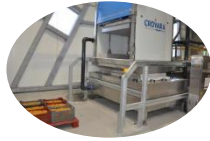
Douchage caisses machine Crovara
